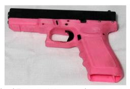
Example 2: 3D Printed Hybrid Firearm (3D printed receiver with metal gun components)
